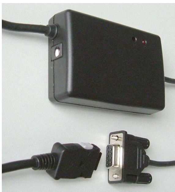
Figure 10: Practical sample of download cable
