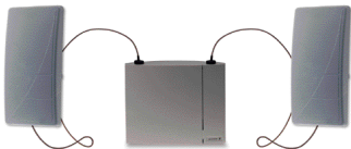
Situation 2 Base station BS340 with directional single antennae
